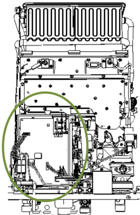
Remove control board Bracket to access
