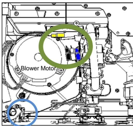
\*Move control board bracket out of way to access outlet thermistor (follow instructions in Section 1).
