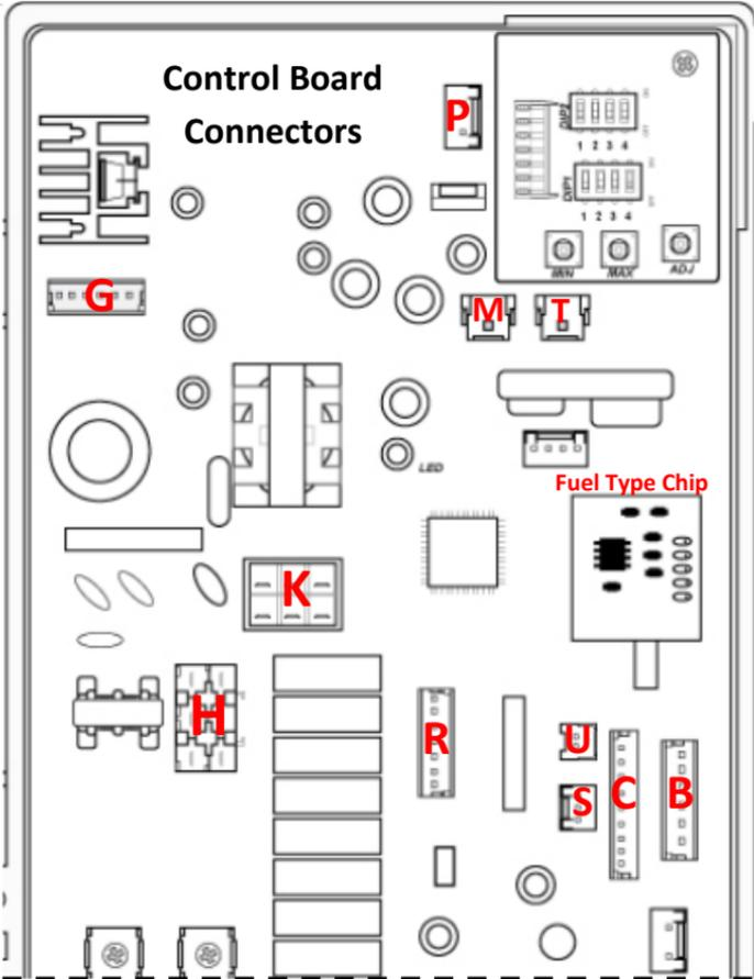
**\*\*\*FUEL TYPE CHIP\*\*\* – When replacing Control Board, you must use the original chip on the new Control Board. New Control Board must be programmed (refer to page 122).**
