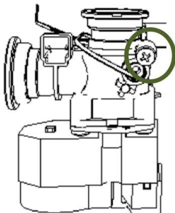
\*Remove Water Bypass & Water Volume valves (follow instructions in Section 7).
