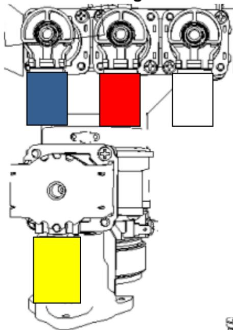
\*Remove 4 Molex connectors on back of gas control valve (highlighted in corresponding wire color).
