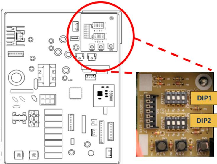
Locate the two DIP switches at top right of Control Board. Switch labeled DIP2 is the bottom switch. Altitude adjustments must be performed on DIP2 ONLY.
