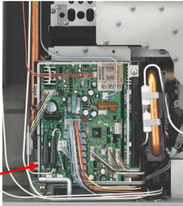
Locate & separate Blue Molex (located near blower motor). Check resistance across White wires on female end of Molex:
