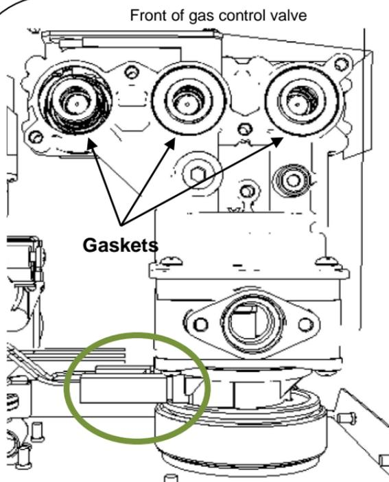
\*Remove 2 Molex connectors and clear tube on left side of gas control valve (circled in green).
