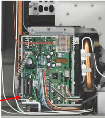
Locate & separate Yellow or Green Molex (located near blower motor). Check resistance across White wires on female end of Molex:
