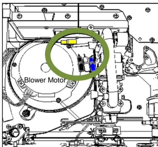
\*Move control board bracket out of way to access WHITE Molex for inlet thermistor (follow instructions in Section 1).
