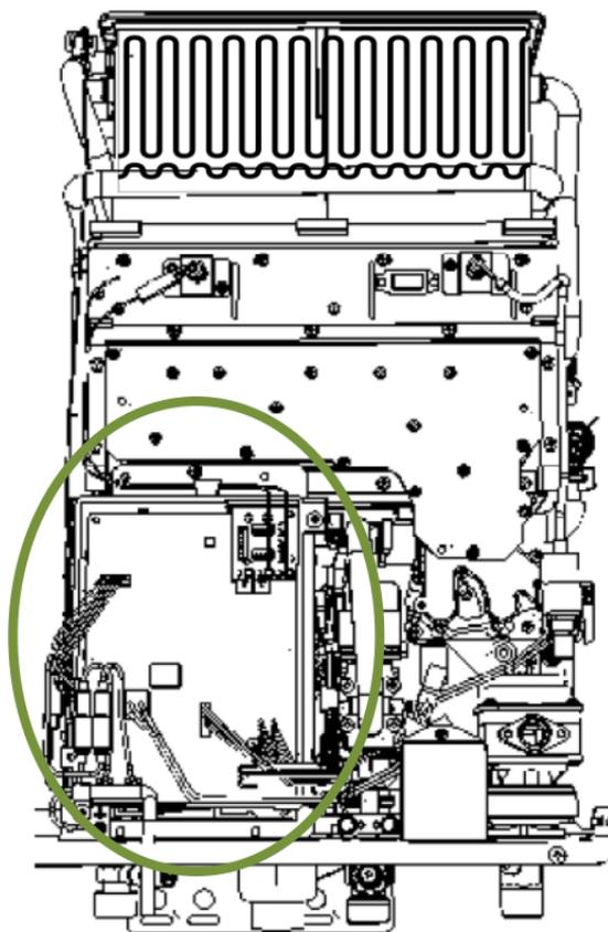
Remove control board Bracket to access inlet thermistor.
