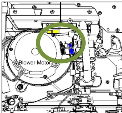
\*Move control board bracket out of way to access Molex for Heat Exchanger thermistor (follow instructions in Section 1).
