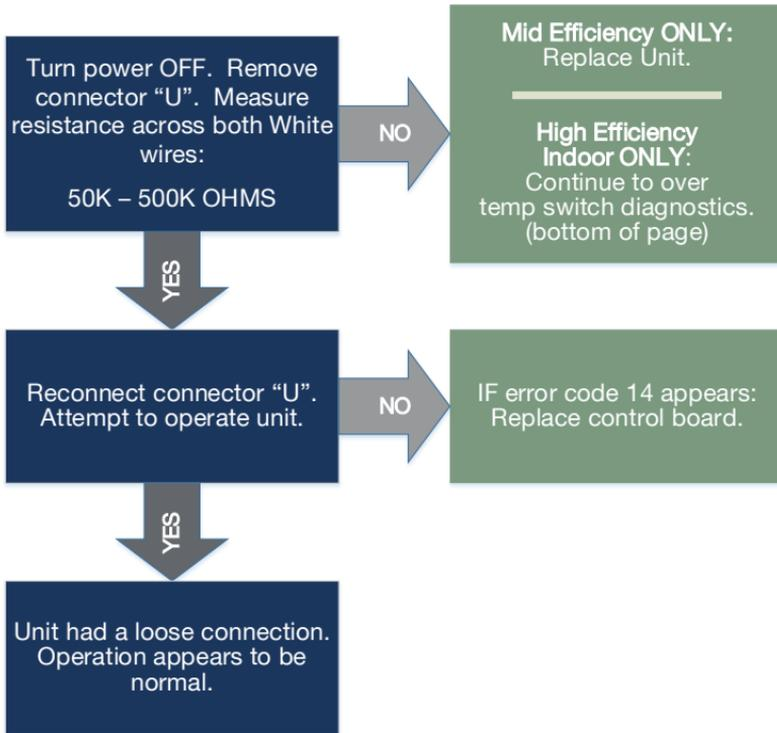
**Over Temp Limit Switch - High Efficiency Indoor (Condensing) ONLY:**
