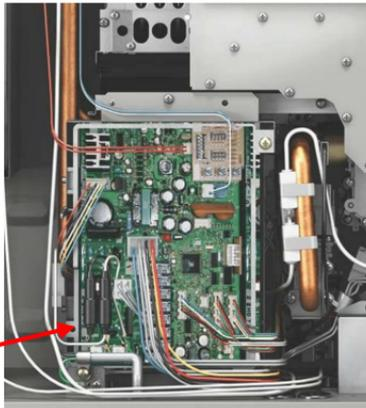
Locate & separate Black Molex (located near blower motor). Check resistance across White wires on female end of Molex:
