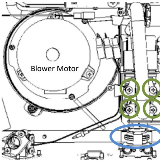
\*Remove 4 screws holding compression fittings in place & remove metal tabs.
