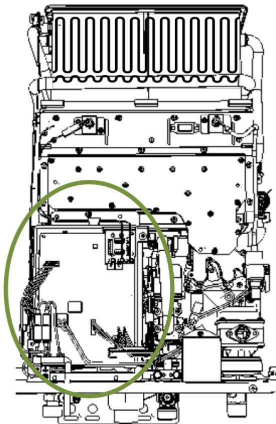
Remove control board Bracket to diagnose and/or replace ambient thermistor.
