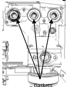
**IMPORTANT:** During reassembly: Make sure ALL 3 gas control valve gaskets are in place.
